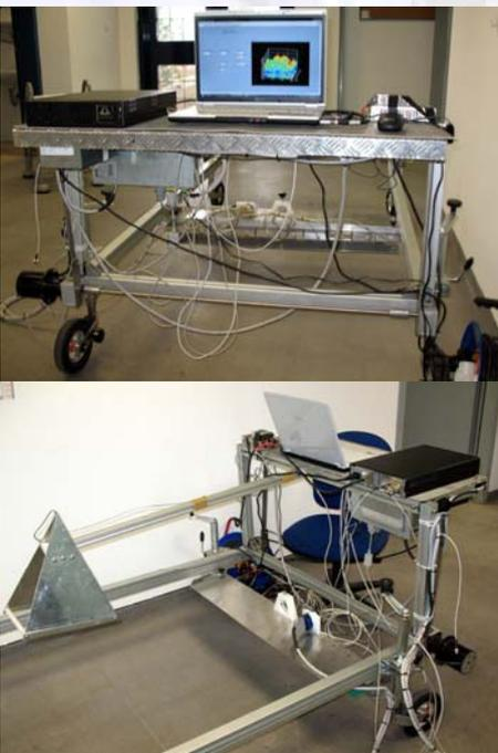
Figure 4. Photos of the GPIR System. In the first photo, the User Interface can be discriminated, while at the photo below, the procedure of measurements is presented
