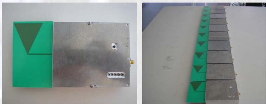
**Figure 3.** Photo of the antenna/receiver and the whole receiving unit by putting 10 separate receiving modules in a row
